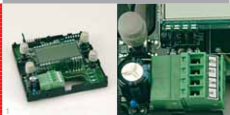
1 ► Internal electronic details of the K481 1 thermostat
